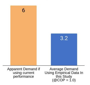
\*Watts/SF of apparent heating demand = Typical Fossil Fuel Heat slope \* boiler efficiency \* 60 HDD / 24 Hours / 3.412Btu/W
