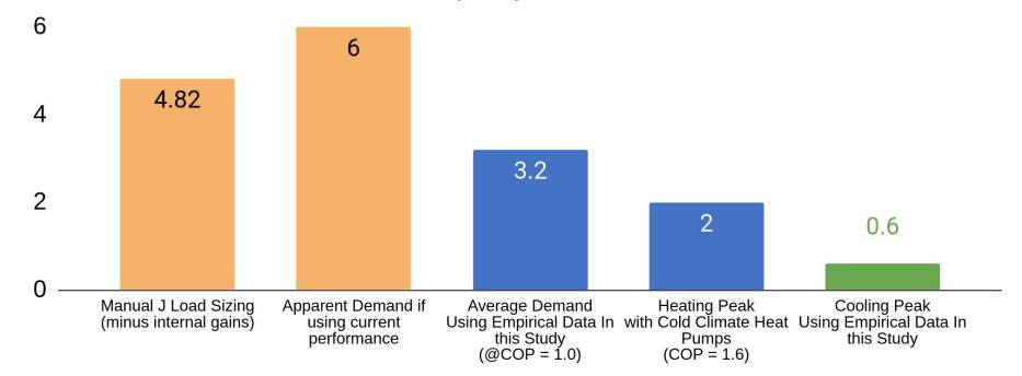
\*Watts/SF of apparent heating demand = Typical Fossil Fuel Heat slope \* boiler efficiency \* 60 HDD / 24 Hours / 3.412btu/W
