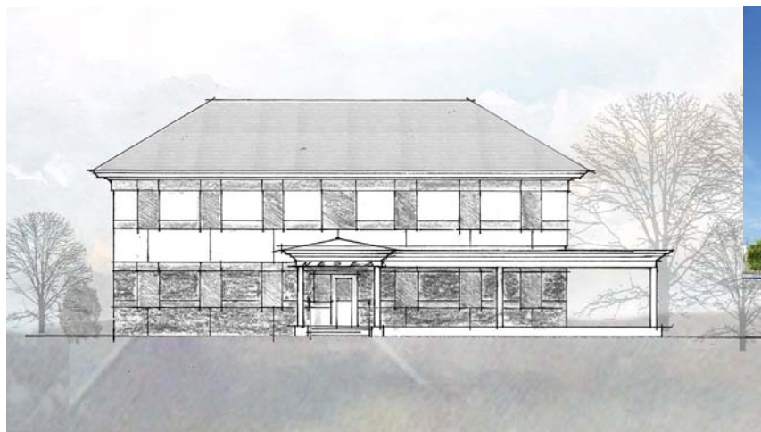
Preliminary Front Elevations using Hardi Panel cladding, and showing an option of a future porch with an entry ramp.
